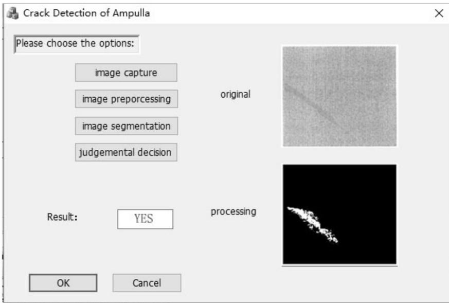
Fig. 6. Results of glass bottle crack detection system
